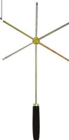
This item is used for comparing the thermal conductivities of aluminum, brass, steel, nickel, and copper. The five radial spokes are attached to a brass hub. Each rod is marked with the metal name on the hub. There are notches in each rod to hold a wax pellet. The unit comes assembled and with a supply of wax. Includes activity guide. Shipping weight: 4.45 oz., dimensions: 14" x 7" x 1".
