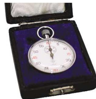
This is a top-quality, precision, single action, mechanical stopwatch. It features a stainless steel spring and 13-jewel movement. The dial face is marked 0-60 seconds x 0.2 seconds and the minutes dial reads to 30 minutes. The watch is housed in a felt-lined wooden storage case.
