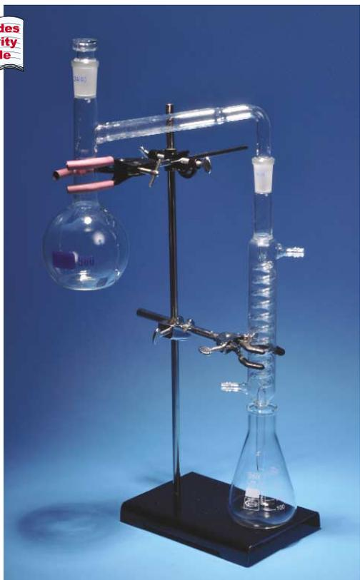
Complete distillation apparatus.
