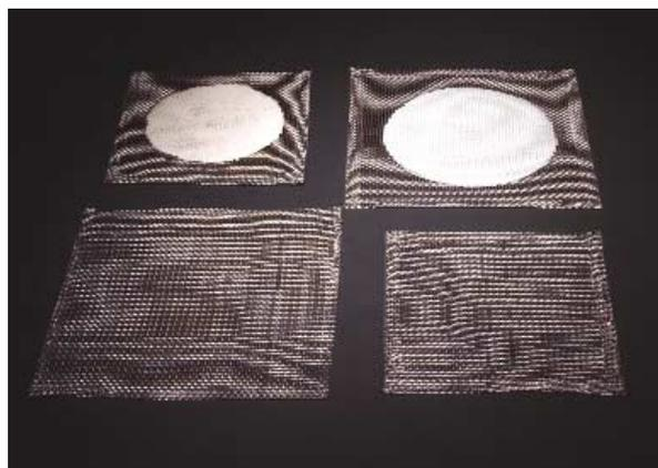
Iron wire gauze (24 SWG/10 Mesh) with ceramic coating at the center. Contains no asbestos. Sold as packs of 10.
