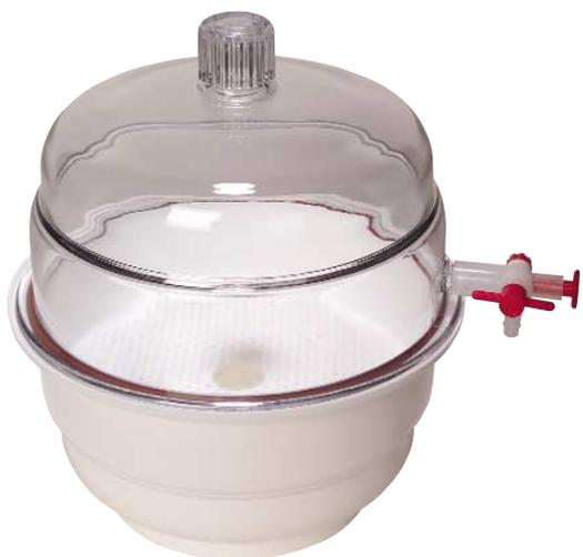
These autoclavable desiccators are made of polypropylene (PP) and polycarbonate and can hold vacuum up to 740mm Hg for 24 hours without any greasing. The PP stopcock has a self lubricating PTFE plug that works to create the vacuum, shut it off and release it. Autoclavable at 120° C for 15 minutes. Non-vacuum (Plain) desiccators are physically the same as vacuum desiccators. Only difference is the absence of stopcock. Grease should be applied on the flanges to make it air-tight.
