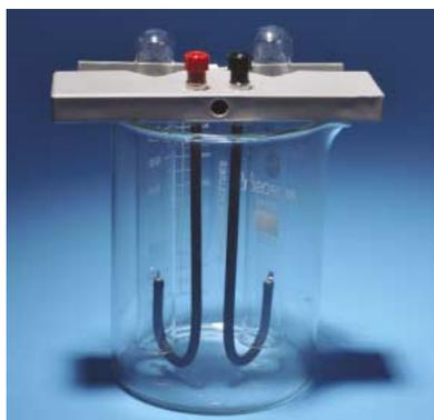
This is a simple and economical type of electrolysis apparatus. Platinum electrodes are attached to insulated connecting rods which are attached to binding posts mounted on a non-conducting support. The support rests across the top of a battery jar (not included) and has two clips that each hold an inverted test tube. Available in two versions, with or without a beaker. The unit operates on a user-supplied 6V battery or 10V DC power supply.
