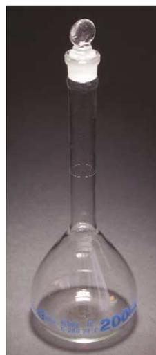
Volumetric Flask with Glass Stopper
