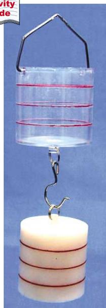
This new model has a much larger capacity (100ml) than the traditional aluminum model (22ml) for higher accuracy and easier operation. Also, both the cylinder and the cup have marked divisions which allow the students to repeat the experiment with different volumes. The cylinder is made of white nylon. This item requires a 200g spring scale, an overflow can and a beaker (not included). Includes activity guide.
