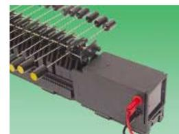
Motor powered eccentric driver can create traveling or standing waves.
