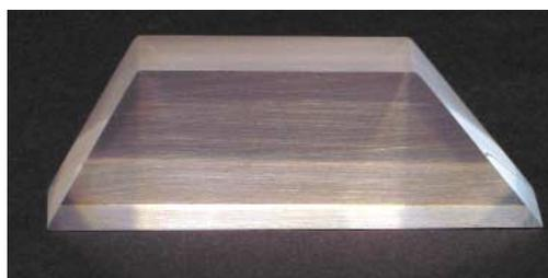
Clear Acrylic trapezoid, with one flat surface frosted to enhance visibility. Bases are 89mm, and 40 mm. Faces measure 47mm and 35mm.
