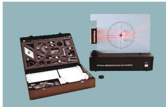
Comprehensive set of equipment with built-in He-Ne laser. Top quality optical glass components allow over 75 experiments in geometric and physical optics.
