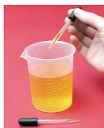
Straight pipettes with glass tube and tapered rubber bulbs. About 70 mm long with 2 ml capacity.
