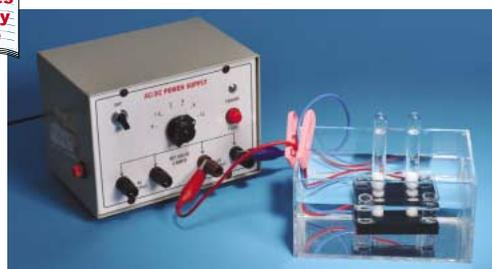
This easy to set up, inexpensive device was designed by teachers in order to collect the correct proportions of hydrogen and oxygen from the electrolysis of water. Its unique design helps correct issues such as falling test tubes perched over unsteady electrodes and gases escaping due to poor alignment.
