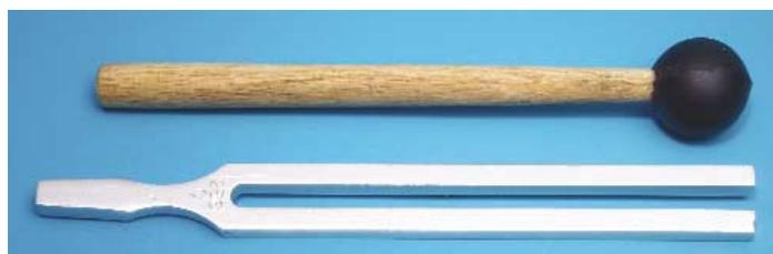
Discover the science of music with the Tuning Fork and Striker Set. The 256Hz tuning fork is made of high-quality aluminum alloy and has been accurately calibrated. A rubber hammer striker for sounding the tuning fork is included. The resonance frequency is stamped on the tuning fork.
