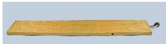
Economical version of the traditional wood inclined plane. 80 cm long x 12 cm wide. Made of MDF. Includes adjustable-angle pulley and a 14mm diameter cross hole for support rod.
