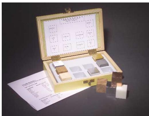
The set includes one each of acrylic, oak, pine, poplar, steel, aluminum, copper, brass, nylon, and PVC cubes. The set of 1" cubes is packaged in a wooden storage box. An economy version, DCSET4, consists of one each acrylic, pine, nylon, and aluminum cubes packaged in a poly bag.
