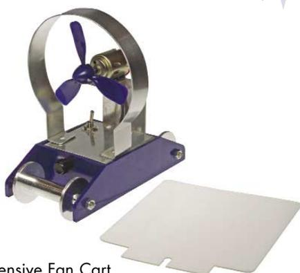
A basic, inexpensive Fan Cart powered by two AA size batteries (not included) demonstrates Newton's principle of action and reaction. The batteries are contained in the removable power unit and the fan is controlled by a switch. The propeller delivers a thrust of about 88mN, accelerating the cart at  $0.4 \text{ m/s}^2$ . A transparent plate can be attached to show the effect of reversing the airflow. Includes activity guide.
