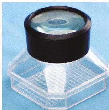
Rugged, clear plastic viewer with 5mm squares on the bottom for easier specimen measurement. The top has a 2.5x glass lens. **Suitable for ages 8+.**
