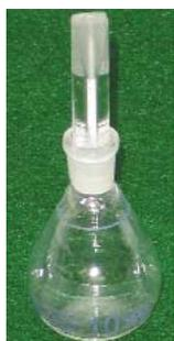
These uncalibrated specific gravity bottles are excellent for determining the specific gravity of liquids. The borosilicate bottles have a ground stopper joint for a precision fit. Available in 10 ml or 25 ml sizes.
