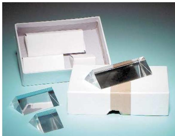
Constructed of clear acrylic with highly polished surfaces, these prisms are ideal for projecting a clear, sharp spectrum. Set of Right-Angled prisms consists of 25mm, 50mm, and 75mm long prisms.
