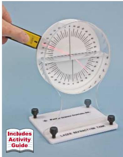
This product effectively demonstrates the laws of reflection and refraction. The 16cm diameter acrylic water tank has a 360° scale and a movable arm carrying a laser activated by a momentary switch. The sharp beam of light produced by the laser can be adjusted to pass the center of the scale. Batteries and an activity guide are included.
