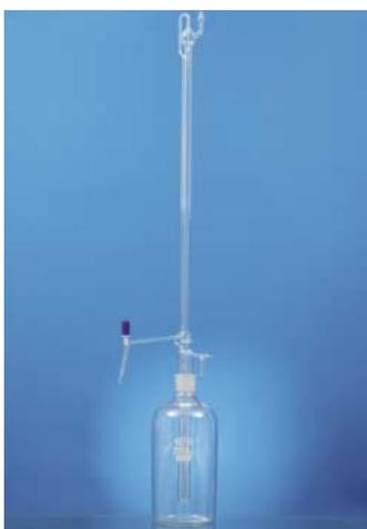
Self-zeroing automatic burette that is mounted on a reservoir with a PTFE needle valve stopcock (screw type) and rubber bellow.
