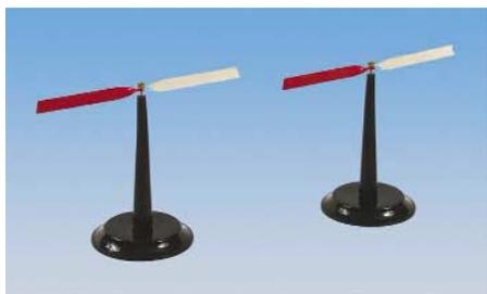
Two 14-cm long magnetic needles with colored poles are mounted on plastic stands with needle bearings. Use individually as a compass or as a pair to show attraction and repulsion.
