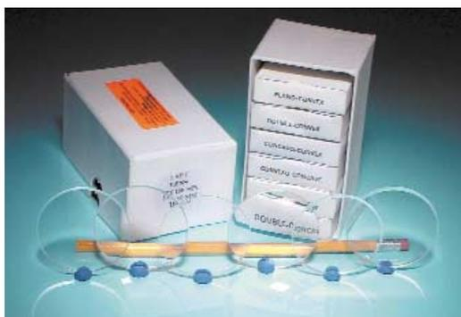
The set contains 6 lenses, one each of double convex, plano-convex, concavo-convex, double concave, plano-concave, and convexo-concave lenses. Comes in a reusable cardboard storage box.
