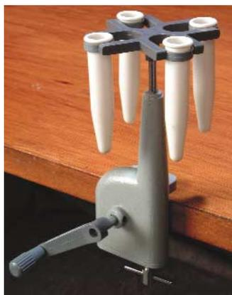
This hand-driven centrifuge comes with a table-mounting clamp. Features a painted metal body, and metal head. Comes complete with 4 each aluminum shields. Easily dis-assembles for storage in specially designed foam box. Crank is geared to head at 16:1 ratio. A crank rate of 12 turns in 10 seconds yields a head speed of 1152 rpm.
