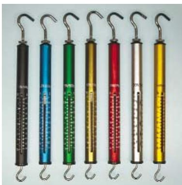
Constructed of anodized aluminum, with steel hooks, this spring scale is extremely durable and designed for long-term use. Available in 7 sizes.
