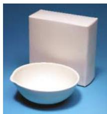
These glazed evaporating dishes can withstand temperatures up to 1050°C. Each dish is individually packed.
