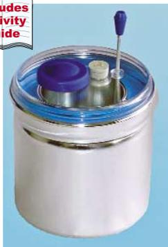
This calorimeter consists of two nested aluminum cans separated by a 1.7cm thick Styrofoam liner and a clear molded plastic lid with a filler cap. A plastic insulator ring protects the Styrofoam insulation against damage and liquid spills. The inner reservoir has a capacity of 150ml. A thermometer stopper and an insulated stirrer are included. Includes activity guide. Shipping weight: 0.5 lb., dimensions: 7" x 4" x 4".
