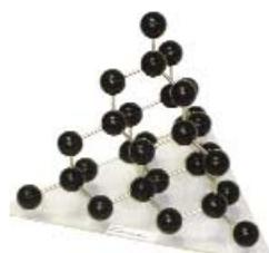
A ball-and-spoke structural model of the diamond crystal form of carbon, permanently mounted on a clear triangular acrylic base. It contains 30 balls, each 22 mm in diameter. Overall dimensions: height 20.5 cm, base side 25.5 cm.
