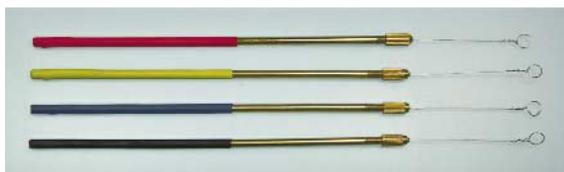
Our inoculating loop features a 8" long solid brass insulated handle, with a non-calibrated 26 gauge nickel-chromium wire loop approximately 5mm in diameter. Now available as a set of 4, with color-coded handles for easy identification.
