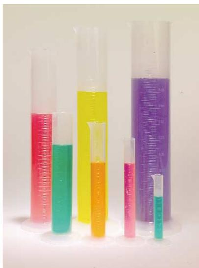
A convenient set of 7 graduated polypropylene cylinders in sizes 10ml, 25ml, 50ml, 100ml, 250ml, 500ml, and 1000ml. Shipping weight: 1.75 lbs, dimensions: 15.5" x 10" x 4".
