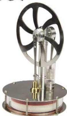
This economical Stirling Engine runs by exploiting the heat flow generated by the small temperature difference between room temperature and a cup of hot water or ice. It is a classic illustration of converting heat energy into mechanical work using a thermodynamic cycle. The engine runs at about 150rpm when used with cup of hot water. Additional information available upon request. Includes activity guide.
