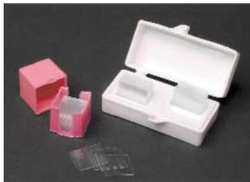
Made of quality, non-corrosive glass. The 22 x 22mm sized coverslips are available in thickness #1 or #2.
