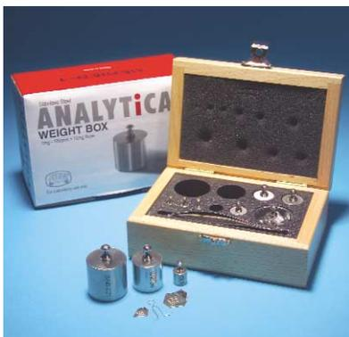
Good quality weight set contains 9 weights (1 each of 1g, 5g, 10g, 50g and 100g sizes, and 2 each 2g and 20g sizes) plus a set of 1 to 500 mg fractional weights and a 5mg rider and forceps, in a wooden storage box. Weights are made of polished stainless steel and each weight is inscribed with its capacity.
