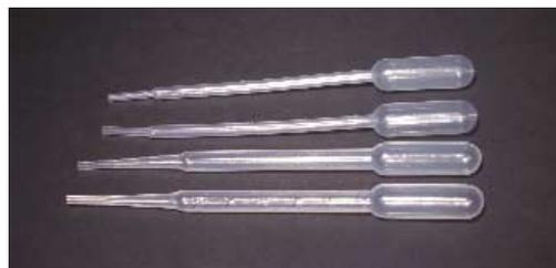
Polyethylene dropping pipettes are graduated, and can be easily rinsed and re-used. Offered in 1ml and 3ml sizes; additional sizes can be special ordered.
