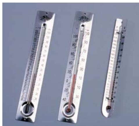
Glass thermometer mounted on aluminum back. Thermometers are filled with approximately 3 grams of Toluene mixed with red color.
