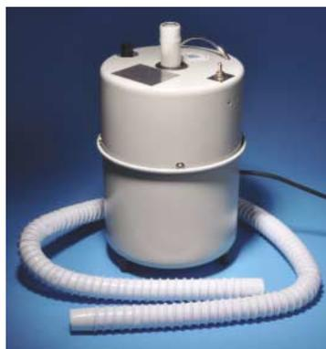
This low noise (<58dB) air source is an ideal accessory for air tracks, air tables, and other pneumatic equipment in physics labs. The 250W motor produces a clean air output with a flow rate of 35 m<sup>3</sup>/hour at a 0.70 kPa overpressure.
