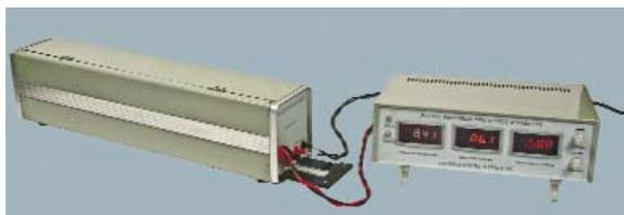
Set of equipment for studying the photo-emission of a mixed alkali photocathode. Precise, stable illumination and bias control for excellent results.
