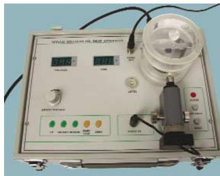
Classic Oil Drop Experiment for measuring the electron charge. Features double draft shield system, CCD microscope camera and computer control for the experiment and evaluation.
