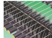
Pendulums are independently suspended on a common base and coupled together by long, light springs.
