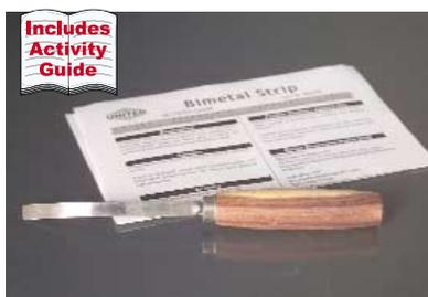
A quick and easy tool for demonstrating thermal properties of matter. Bar is bi-metallic and has a wooden handle attached. When heated, the bar bends dramatically. Includes activity guide. Shipping weight: 0.25 lbs., dimensions: 9" x 1" x 1".
