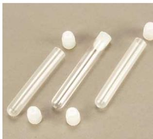
Available in both polypropylene and polystyrene. The polypropylene vials are designed for use with common acids, alkalis, and solvents at room temperature. The polystyrene vials are designed for use with mild bases and weak acids.
