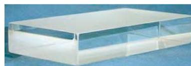
Rectangular glass block with two frosted sides, 114 mm x 63 mm x 19 mm.
