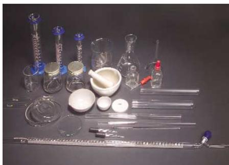
Quality glassware assortment for use in general science, or chemistry laboratory. Kit includes following items, and is designed for use by 2-4 students. Shipped in a re-usable storage box. Shipping weight: 15 lbs., dimensions: 33" x 11.5" x 5.5".
