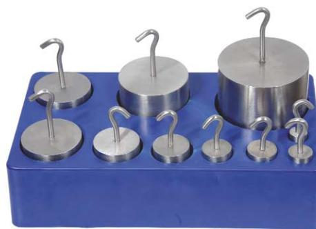
Individually calibrated weights made of high quality stainless steel. Both sets come with a sturdy plastic storage block. Set of 9 includes 1 each of 5g, 10g, 50g, 100g, and 500g, plus 2 each of 20g and 200g weights.
