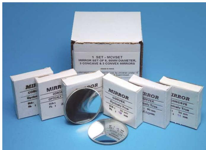
A set of six glass spherical mirrors with back surface silvering. Includes three convex and three concave mirrors, all of 50 mm diameter. Focal lengths are 50 mm, 100 mm, 200 mm, -50 mm, -100 mm and -200 mm.
