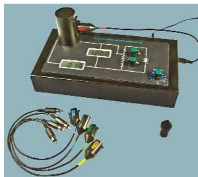
A precision device for measuring Planck's Constant and the work function of electrons in cesium. **See full description on page 45.**
