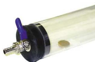
An economical version of a classic device! It demonstrates that all objects experience the same gravitational acceleration and fall at the same speed in a vacuum, but in air the air resistance slows down some objects more than others. Features a disc and a feather in a tough, clear, plastic tube, 90cm long and 4.5cm diameter, with rubber end caps and hose cock for connection to any standard vacuum pump (not included.) Includes activity guide.
