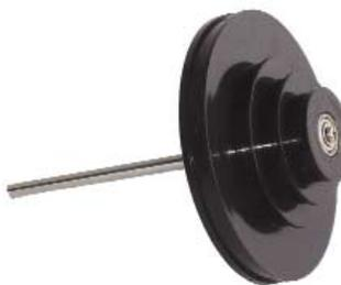
This is a classic device for demonstrating mechanical advantage and the conservation of energy. It consists of a single stepped wheel with four coaxial steps of 35, 50, 65, and 105 mm diameter. The wheel is supported on a steel rod by a ball bearing.
