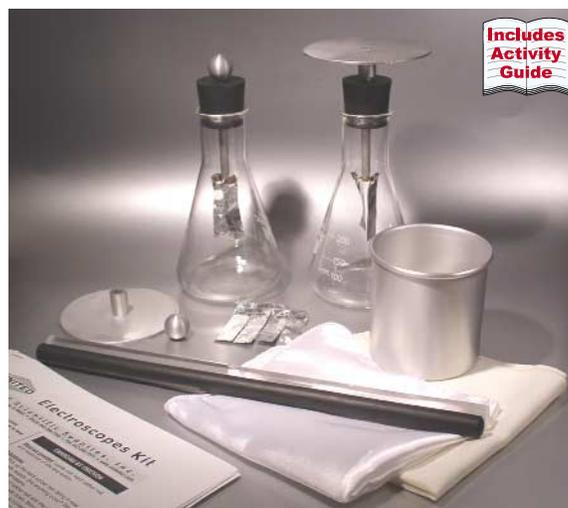
Demonstrate key electrostatics concepts with this kit. Contains everything necessary to construct two flask form electroscopes. Detailed activity guide includes experiments using two electroscopes for positive and negative charge studies, and a Faraday's Pail experiment. Kit includes 2 Glass Flasks, 2 aluminum disc terminals, 2 sets of 4 foil leaves, 2 electrode assemblies, one aluminum can (Faraday Pail), 1 hard rubber rod, 1 silk cloth, 1 acrylic rod, and 1 wool cloth.
