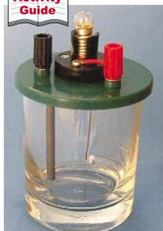
This 3V conductivity tester demonstrates the electrical properties of various liquids. The item consists of a molded plastic lamp socket mounted on a base with 2 binding posts for connecting a wire cord. It comes complete with a bulb and glass tumbler. Includes an activity guide.
