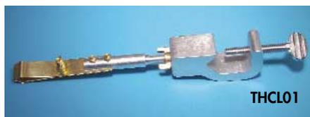
Clamp with Hook can be rotated and locked in any position. Ideal for supporting suspended thermometers, drying tubes, etc.
