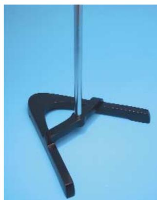
The A-shaped base is made of rugged, cast iron for extra stability. It has 22 cm long legs and features a baked-on black chemical resistant finish. The rod is zinc plated steel, 61 cm long and 12 mm in diameter.
