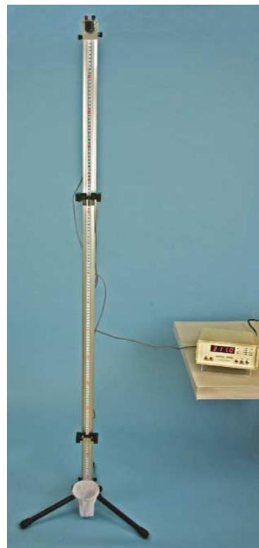
This convenient free fall apparatus for measuring the acceleration of gravity has a 150 cm fall length. It comes with an electromagnetic ball release, a pair of photogates on a long cable harness, two steel balls, a plumb line, a catcher, and an instructional manual. Requires the Digital Timer DTPHG1 (not included). More detailed description available upon request. Includes activity guide.
