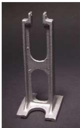
Sturdy support for meter stick demonstration balances and torque experiments. The cast metal support is 18.5 cm high. Requires knife-edge clamps, slotted weights and hangers, and a meter stick.
