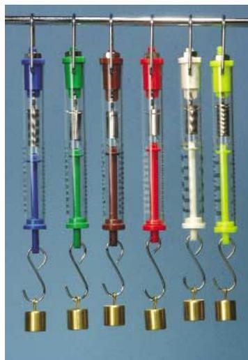
These spring scales feature a clear plastic tube design, and are color-coded. A zero adjustment screw is provided at the top. Overall length is approximately 7".
