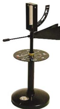
This simple tool measures wind speed and direction. The wind speed range is 0 to 17 meters per second ( $\pm 10\%$ ). The direction indicator is divided into 16 compass points. A built-in compass is provided. Shipping weight: 0.25 lb., dimensions: 9" x 6" x 6".
