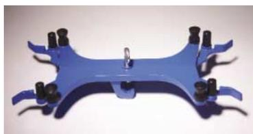
Deluxe Burette clamps are die casted from aluminum and feature black rubber sleeves for firm gripping of burettes. The adjustable clamps hold up to 30mm OD burettes which are held in place by the pressure created by the springs. For use with rods up to 19mm diameter.
