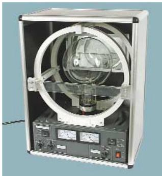
Classic "fine beam tube" set for the visual and quantitative demonstration of electron beam properties and the measurement of  $e/m$ . The compact apparatus has a built-in power supply and is housed in a metal case for easier beam visibility.
