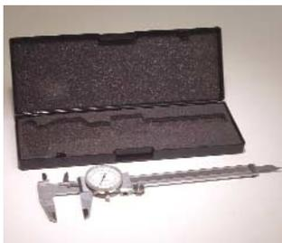
This precision measuring tool is made of hardened steel for precision and durability. It has a range of 150mm and a large, easy-to-read dial with a resolution of 0.02mm. A storage case and instructions are included.
