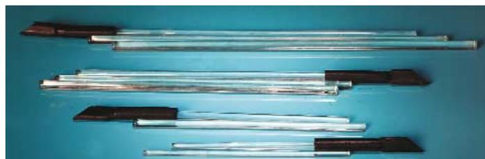
Stirring rods made of soft glass, with both ends rounded.
