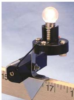
This light source is designed for use with a meter stick optical bench. The 1.5V bulb operates on a single AA battery (not included).
