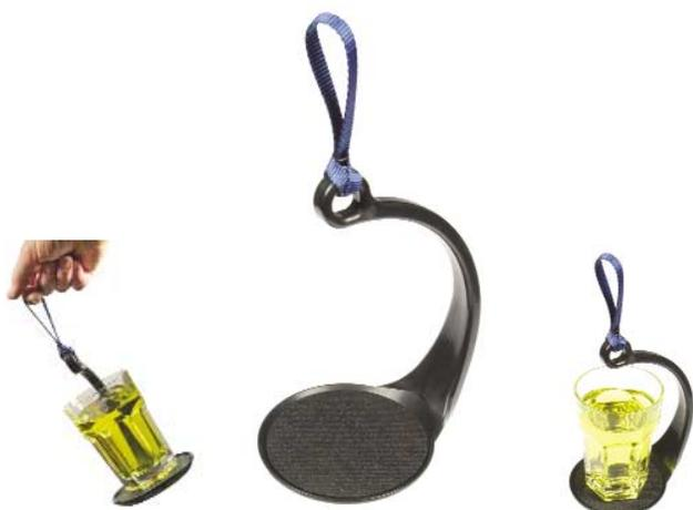
An inexpensive demonstration to intrigue students and challenge their analytical powers! The design of the SpillNot™ uses the principles of Newtonian physics to keep the liquid in the container. The flexible handle and the location of the suspension point above the center of the tray ensure that the forces on the liquid are always directed towards the supporting tray, even when the tray is in motion. **See full description on page 33.**
