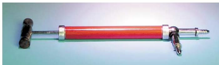
This pump features a steel barrel, steel valve assembly, and a wooden handle. Both in and out ports are equipped with hose connectors, for use with vacuum experiments as well as to generate pressure. Creates vacuum of 20" Hg. Length 14", barrel diameter 1". Shipping weight: 1 lb.
