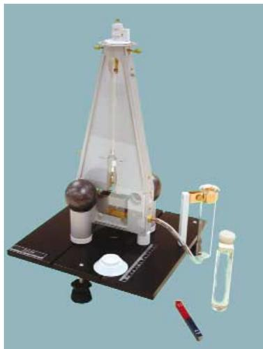
Unique small scale version of the famous Cavendish experiment to verify Newton's Law of Gravity and measure the Universal Gravitational Constant,  $G$ . This unit is remarkable for measuring the tiny value of  $G$  by simple, easily-understood means.
