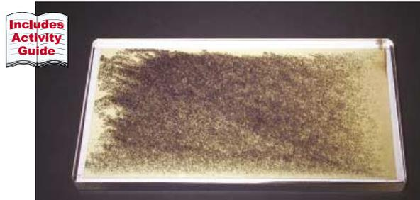
This is a quick and clean way to visualize magnetic fields. The demonstrator is a transparent acrylic case that holds iron filings suspended in a fluid of appropriate viscosity. When it is placed over a magnet, the field pattern can be viewed directly, or it can be placed on an overhead projector for classroom demonstration. Shipping weight: 10.6 oz., dimensions: 8.75" x 4.75" x 0.5".
