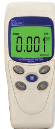
Measure the electromagnetic field radiation intensity that is produced from welding equipment, microwave oven leakage, and other environmental safety concerns
