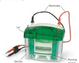
Fig. 2.5. Components of a vertical electrophoresis cell.
