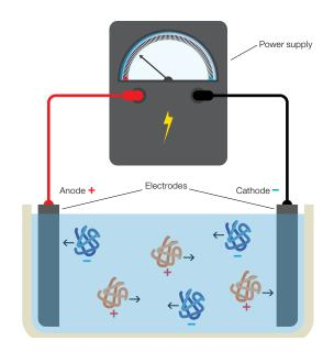
Fig. 1.1. Movement of proteins during electrophoresis.
