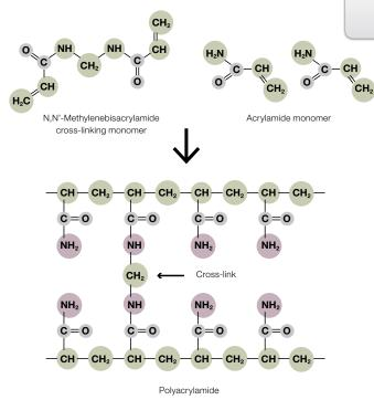
Fig. 4.2. Polymerization of acrylamide monomers and bisacrylamide.
