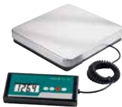
TE150 Stainless steel platform. 150 lb x .2 lb / 70 kg x .1 kg. 6' coiled cord and 1" LCD readout. Runs on adaptor (included) or 6 AA batteries (not included).
