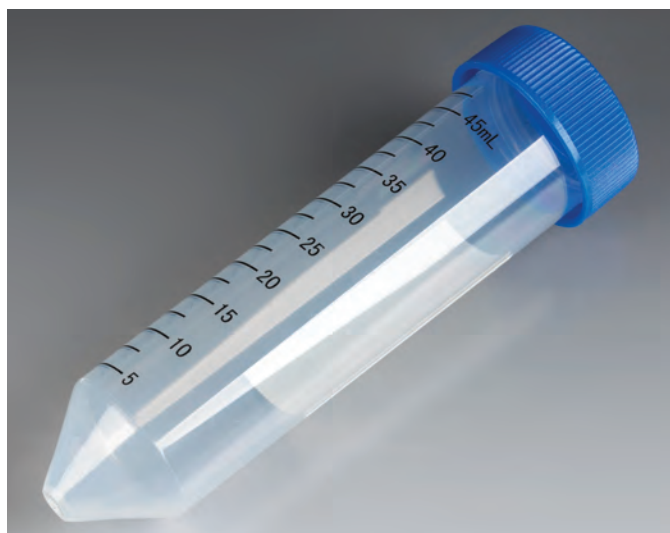
50mL polypropylene centrifuge tube
