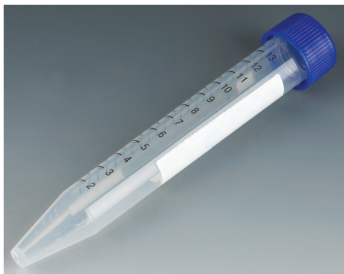
15mL polypropylene centrifuge tube
